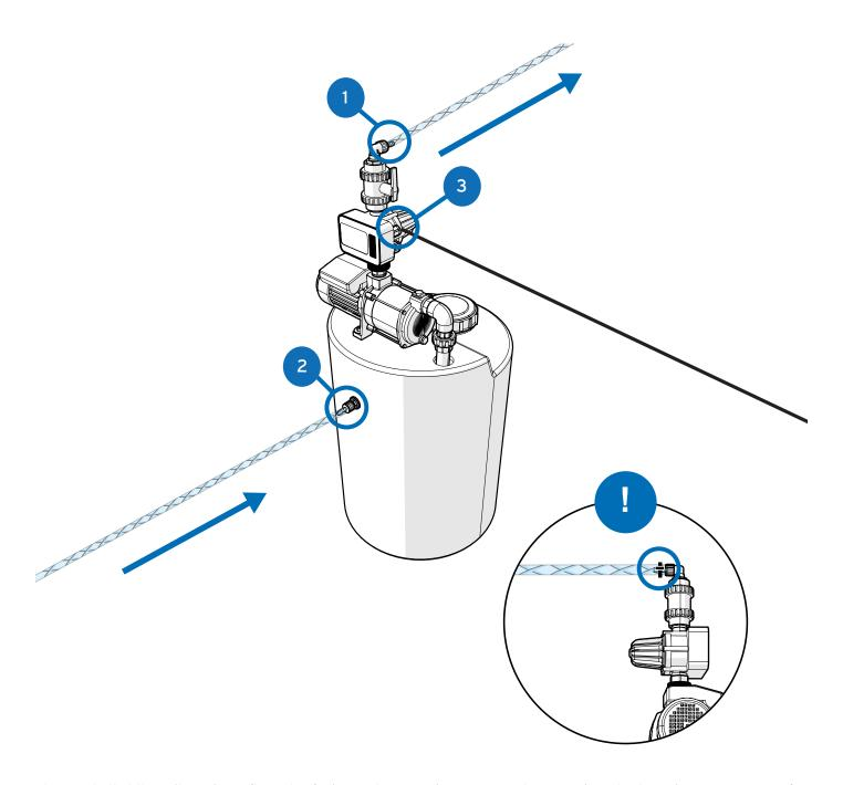
Please note that the unit requires a flow rate of min 68 Fl oz per min - max 339 Fl oz per min and a dynamic pressure range of 28 PSI (min) - to 44 PSI bar (max). A booster tank is recommended whenever a consistent supply is not available.
