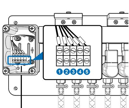
Use a **7x18 AWG** cable for the connection between the control cabinet and the distributor. Connect the distributor to terminal block **X7**. Each terminal connection corresponds to the outlets numbered from left to right, with the number dependent on the order. Below is the wiring diagram for the main unit.
