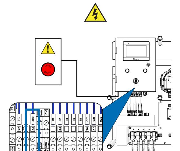
To connect an emergency stop button to your unit, you can use the EXT1 and EXT2 connectors slot shown above in series.
