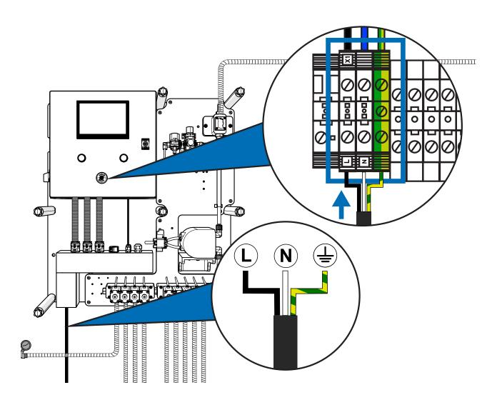
For the power supply of the equipment you must use **3x16 AWG cable**. Insert the cable through the channel located at the bottom left and use one of the cable glands to insert it safely inside the control cabinet. Connect to the terminals identified with **X1** found on the lower left of the connections.
