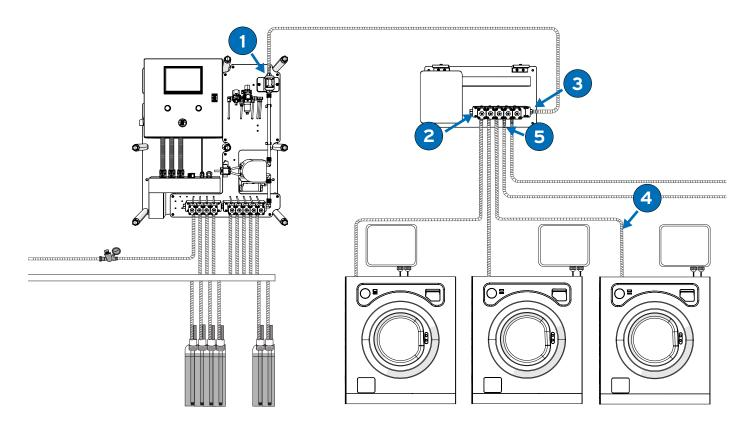
To connect equipment, distributor and washers, use 3/8" ID x 1/2" OD braided PVC pipe and stainless steel clamps.
