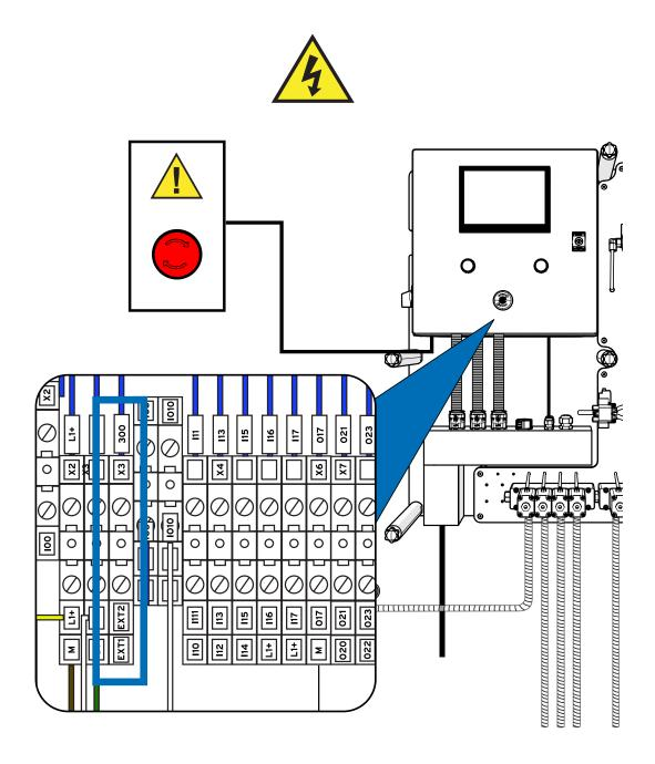
To connect an emergency stop button to your unit, you can use the EXT1 and EXT2 connectors slot shown above.
