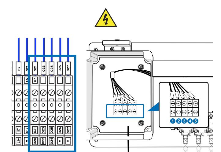
Use a 7x18 AWG cable for the connection between the control cabinet and the distributor. Connect the distributor to terminal block X7. Each terminal connection corresponds to the outlets numbered from left to right, with the number dependent on the order. Below is the wiring diagram for the main unit.
