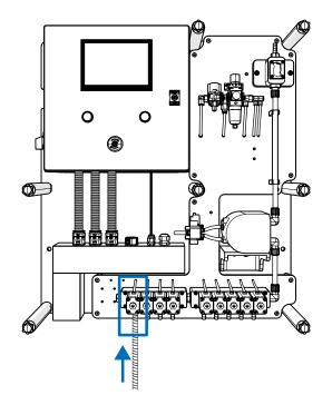
Connect the water supply to the leftmost pneumatic valve on the central panel of the unit.
