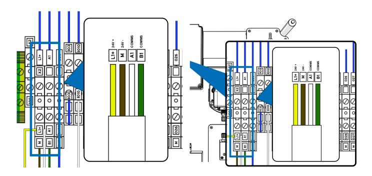
To connect the expanision channel to the unit, connect X2 on the main machine to X1 on the expansion channel.
