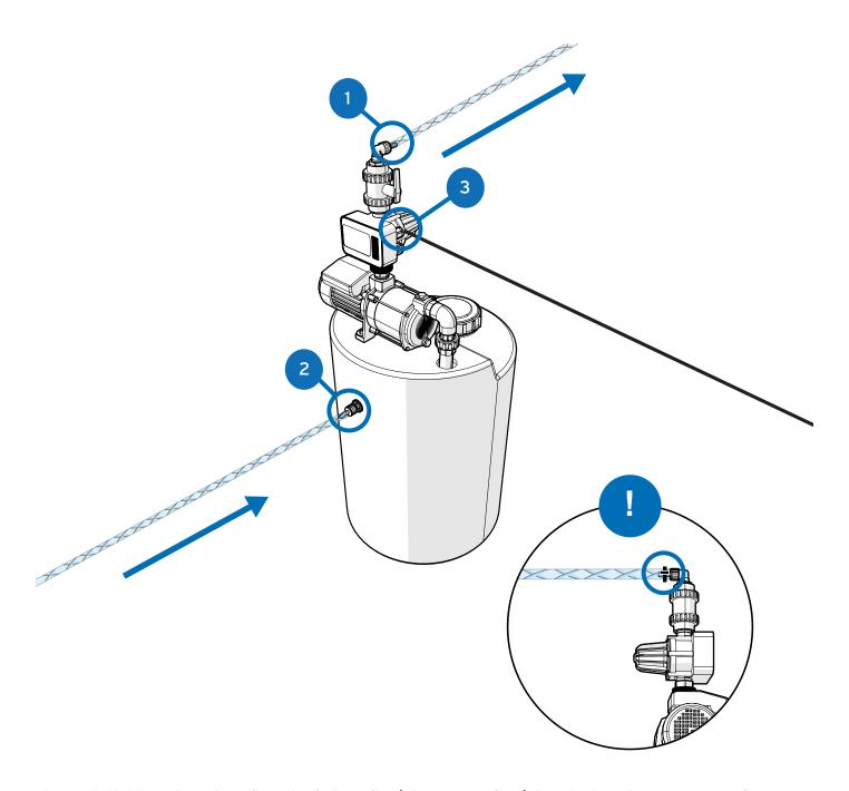
Please note that the unit requires a flow rate of min 68 fl oz/min - max 339 fl oz/min and a dynamic pressure range of 28 PSI (min) - to 44 PSI bar (max). A booster tank is recommended whenever a consistent supply is not available.
