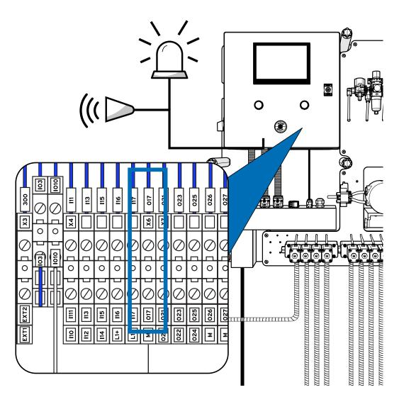
To connect an external alarm or warning light to the system, utilize slot X6 as depicted above.
