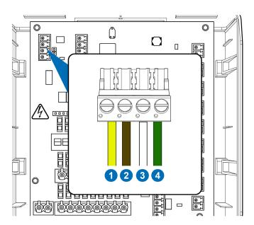
To connect the external communication box to the unit, connect terminal X2 on the main machine to terminal X1 on the communication box. Each communication box can serve up to two washing machines.
