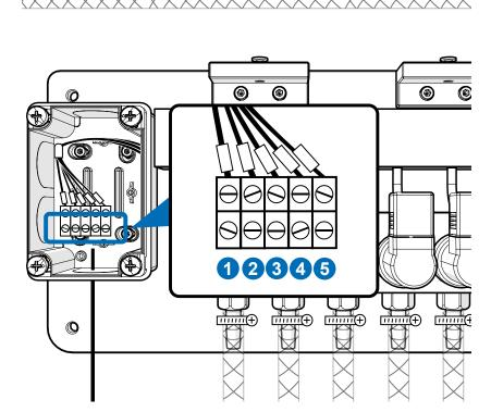
Use a 7x1mm^2 cable for the connection between the control cab inlet and the distributor. Connect the distributor to terminal block X7. Each terminal connection corresponds to the outlets numbered from left to right, with the number dependent on the order. Below is the wiring diagram for the main unit.
