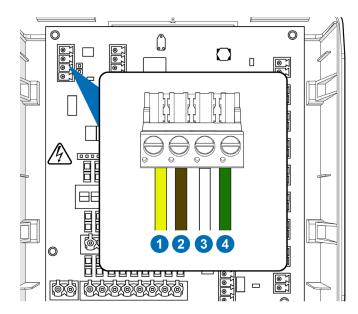
To connect the external communication box to the unit, connect terminal X2 on the main machine to terminal X1 on the communication box. Each communication box can serve up to two washing machines in series.
