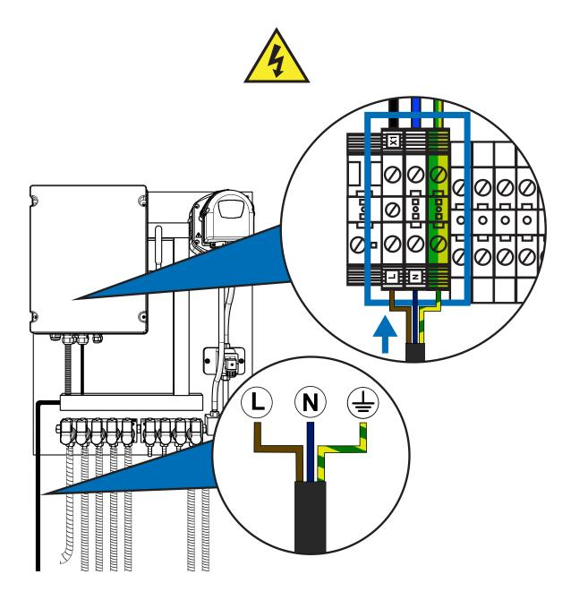
For the power supply of the equipment you must use **3x1'5mm2 cable**. Insert the cable through the channel located at the bottom left and use one of the cable glands to insert it safely inside the control cabinet. Connect to the terminals identified with **X1** found on the lower left of the connections.
